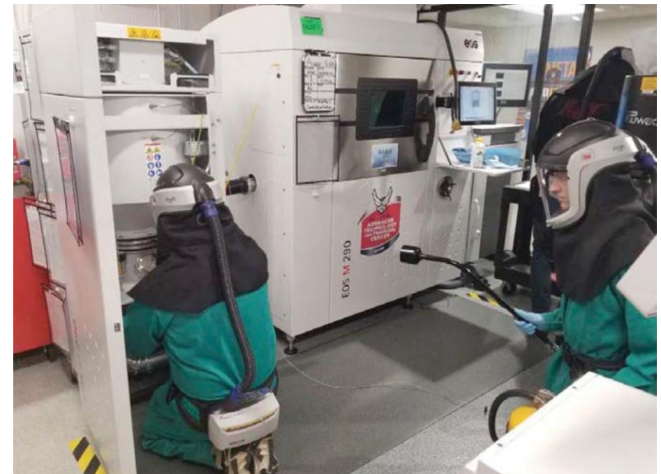
Buddy system for changing large filters which cannot be isolated pre-removal
