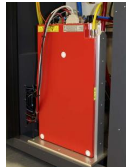
500W ytterbium fibre laser unit – Renishaw RenAM 500M
