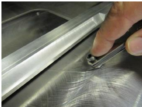
Feeler gauge checking height
