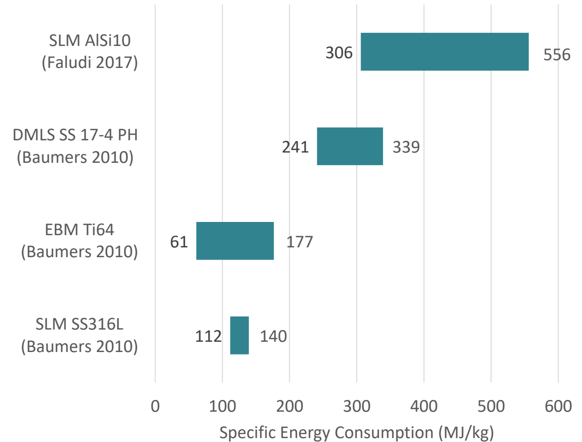
Figure B: Specific Energy Consumption (SEC) of AM processes for different materials [3-7]
